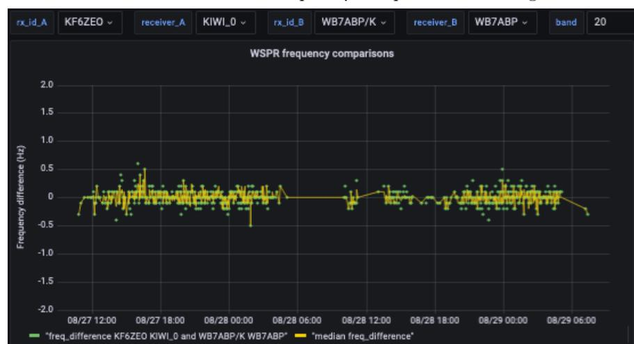
Figure C1. Frequency difference time series over 48 hours for two phase-lock KiwiHDR stations KF6ZEO and WB7ABP on 20 m. The rms difference was 0.13 Hz.
