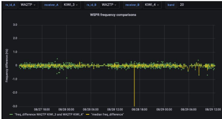
Figure C5. Frequency difference time series over 48 hours between two standard KiwiSDR receivers at WA2TP on 20 m.
