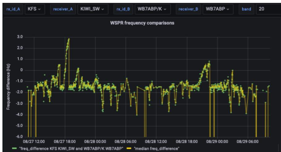
Figure C2. Frequency difference time series over 48 hours for one standard and one phase-lock KiwiSDR stations KFS and WB7ABP on 20 m.
