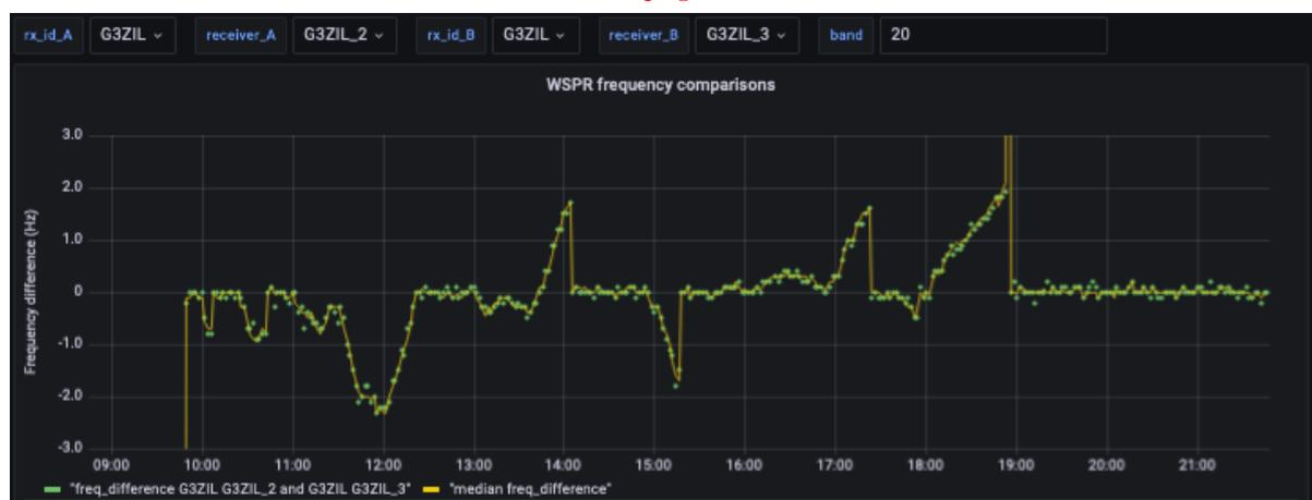
Figure C4. Frequency difference time series over 48 hours between two standard KiwiSDR receivers at one site on 20 m, G3ZIL\_2 and G3ZIL\_3.
