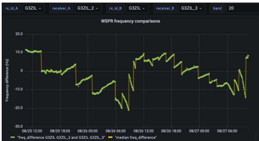
Figure C3. Frequency difference time series over 48 hours between two standard KiwiSDR receivers at one site on 20 m, G3ZIL\_2 and G3ZIL\_3.
