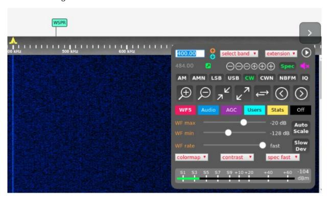
At -104 dBm F2-F1 is 87 dB below total input power for an indicated SHI of -17 + 87 = +70 dBm, input referenced. The amplifier output is 20 dB higher so would be +90 dBm and can be compared to LTC specifications for the part. I have difficulty understanding since there are so many conditions. Schematic for the Kiwi which shows amplifier termination impedances, which appear to be important, is at KiwiSDR schematic.
